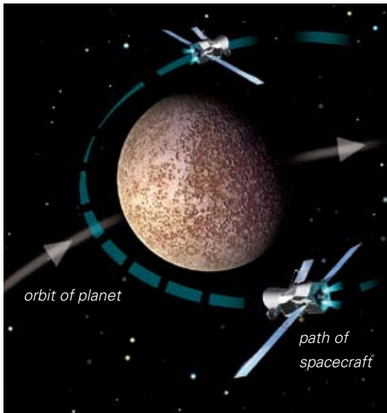
The path of a spacecraft as it performs a slingshot manoeuvre around a planet.
