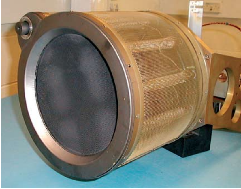
One of QinetiQ's T6 ion propulsion engines ready for tests ...
