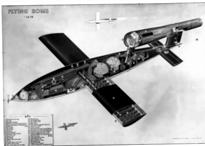
Cut-away diagram of a flying bomb used in the Second World War
