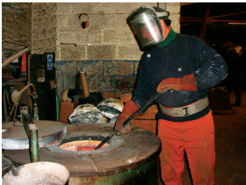
Stirring the furnace to ensure that the mixture is the same all the way through
