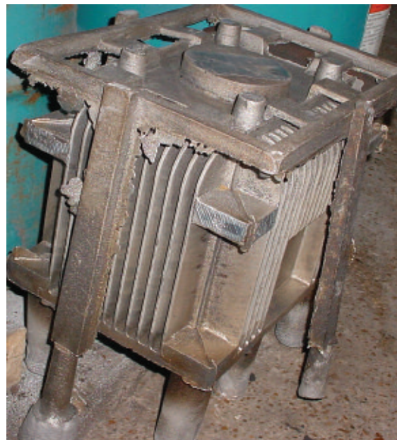
The finished object — ready to have excess metal trimmed off and then cleaned up
