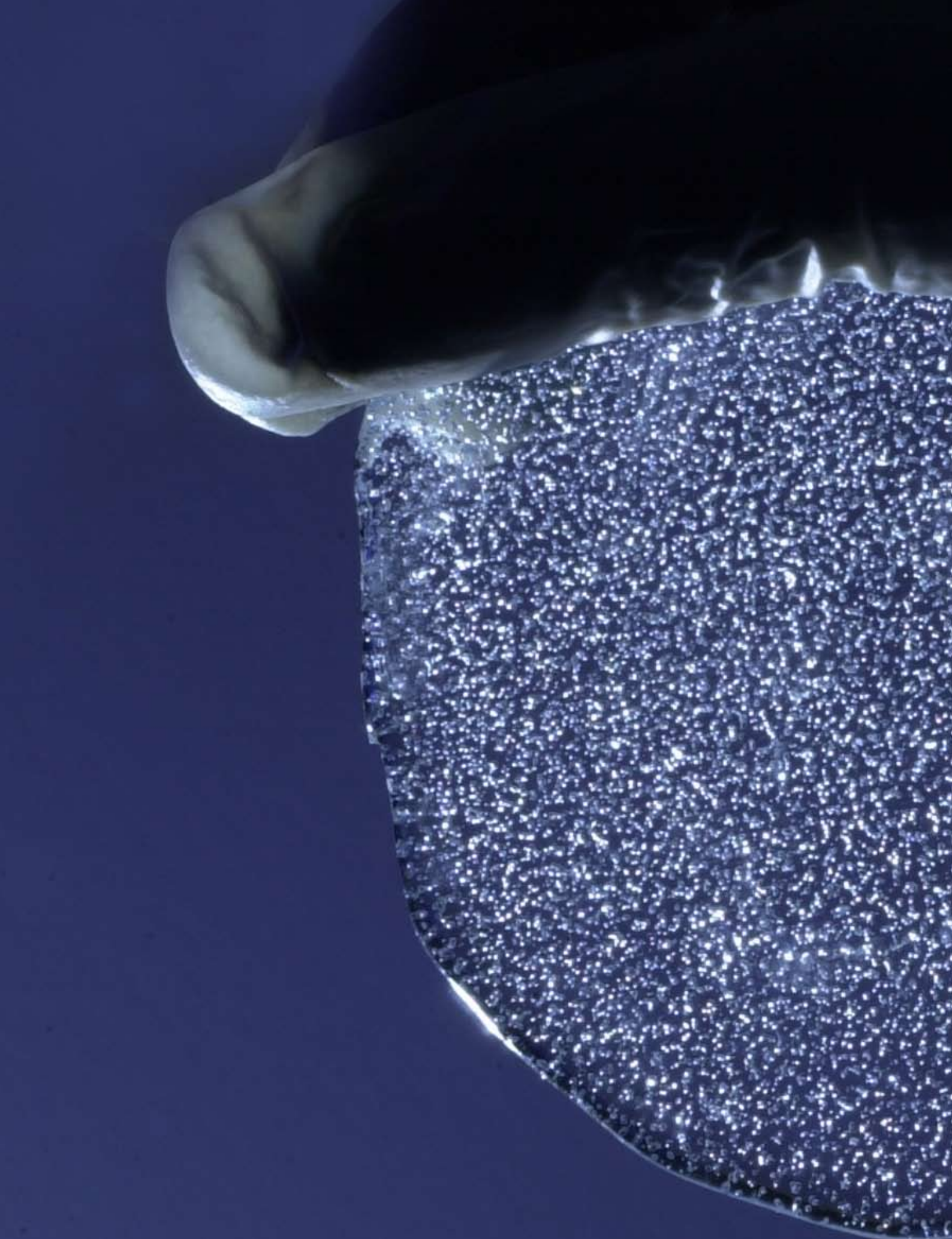
A thin slice of Antarctic ice holds air bubbles, trapped for centuries. Analysing this air tells us how our atmosphere is changing.
