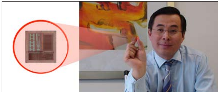
Figure 6 A prototype Application-Specific Integrated Circuit (ASIC) chip for a body-sensing node held by Prof. Guang-Zhong Yang – Imperial College London
