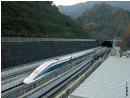
Trains of the experimental Japanese Yamanashi rail link use superconducting electromagnets to levitate them above the track.
