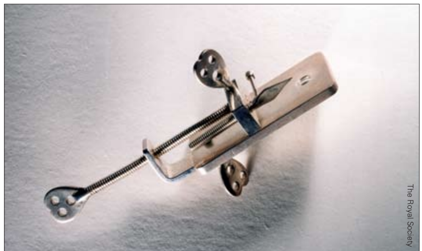
A replica of Leeuwenhoek's simple microscope. Specimens were fixed to the sharp point and viewed through a tiny lens mounted in the small hole.
