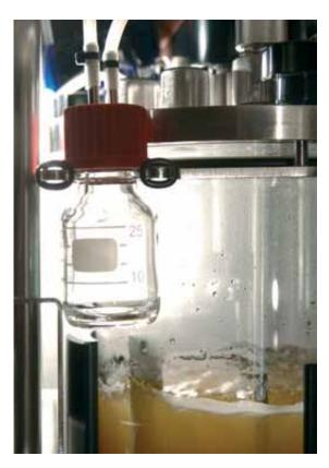
A laboratory fermenter for experiments using bacteria.
