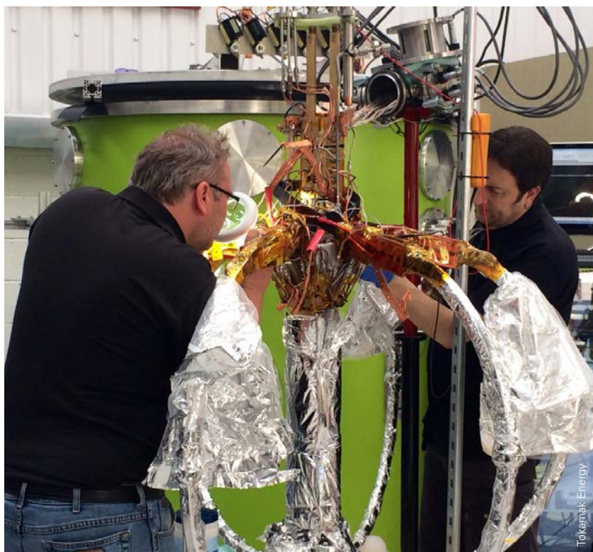
Figure 4 Assembling the high temperature superconducting magnets.
