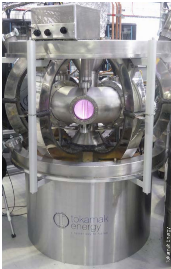
Figure 2 A tokamak with new, high temperature superconducting magnets used by Tokamak Energy. Plasma can be seen in the chamber.
