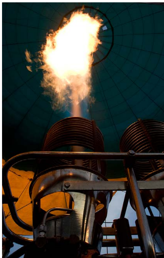
Burning gas to give a hot air balloon greater lift
