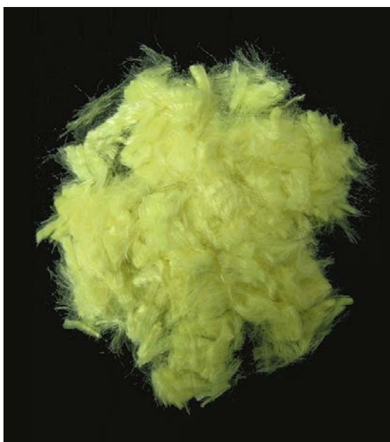
Kevlar fibres – each fibre is about 10 micrometres thick.
