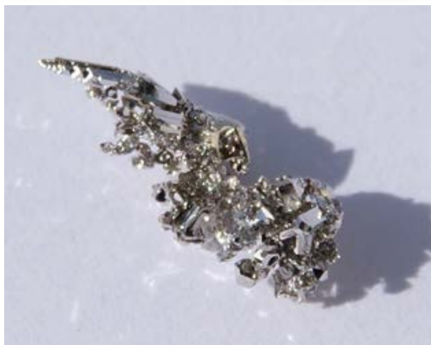
A crystal of palladium with a mass of about 1g and about 1cm in length
