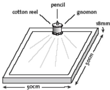
1. You will need 50 X 50 cm thick board (like block board or MDF, 18mm thick); a cotton reel, pencil stub about 6cm long and glue to attach the cotton reel to the board, blank paper that will fit on the board, blue-tack, a compass (fluid-filled type), pencil, and a watch or clock.
