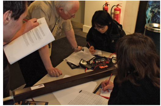
Figure 4 A-level students experimentally exploring the relationship between intensity and distance using solar panels in the context of electrical power for spacecraft
