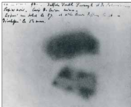
The photographic plate produced by Henri Becquerel to demonstrate the existence of radioactivity
