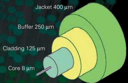
The optical fibre through which light travels is as thin as a human hair.
