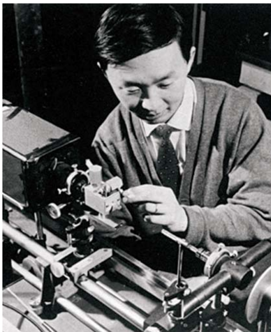
Charles Kao at work in his lab in the 1970s. He is using an optical bench with a laser (left) to shine light through a variety of test materials.
