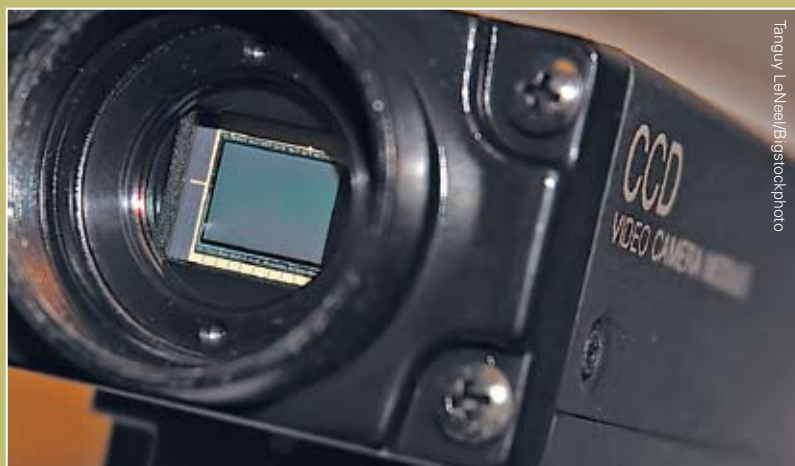
A video camera – the lens assembly has been removed to show the CCD.
