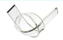
**Cold-forming plastic is a smart material** that can be shaped by hand at room temperature.
