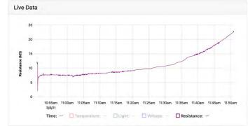
Resistance increasing over time. This shows that moisture levels are decreasing in the soil.
