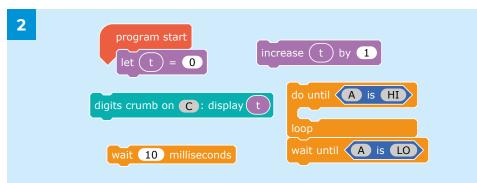
Use these blocks to create a program that counts up from zero every 10ms and displays the value until the button connected to A is pressed.
