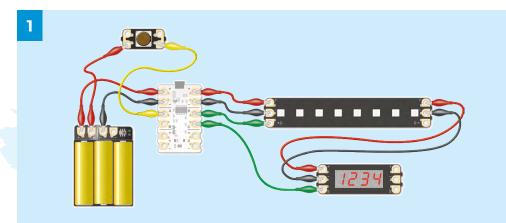
Connect the Crumble, Digits Smart Crumb, Sparkle Baton (optional), batterypack and push-button switch.
