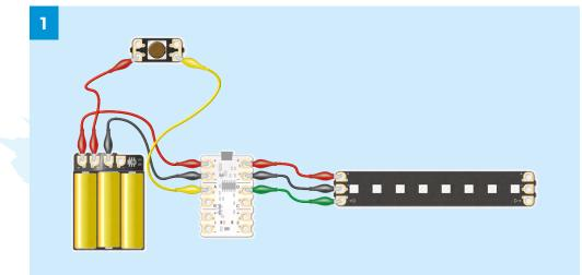
Connect the Crumble, Sparkle Baton, battery-pack and push-button switch.
