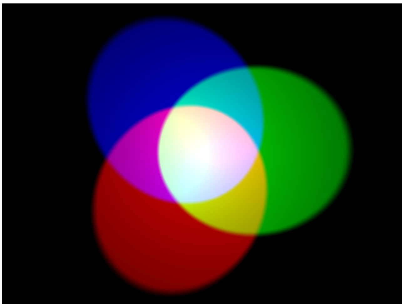
Figure 5: Red, green and blue light is directed onto a screen. Where the lights overlap, different colours can be seen. Where all three overlap, white light is produced. By adjusting the brightness of the different lights, different shades can be produced.
