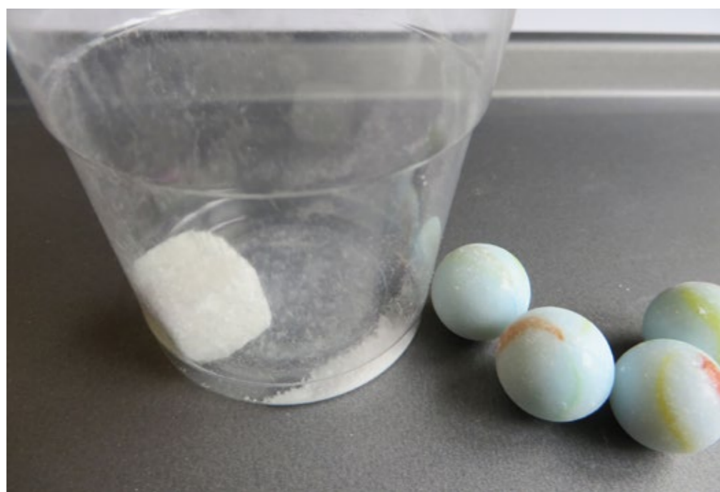
Image shows damage to sugar cube after shaking with marbles in a cup
