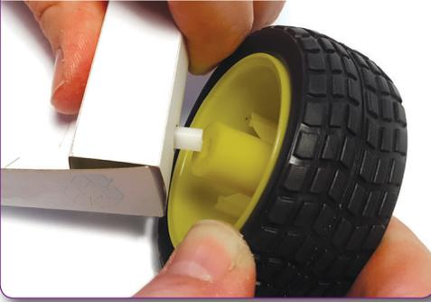
Press the wheels on whilst supporting the back of the gearboxes.
