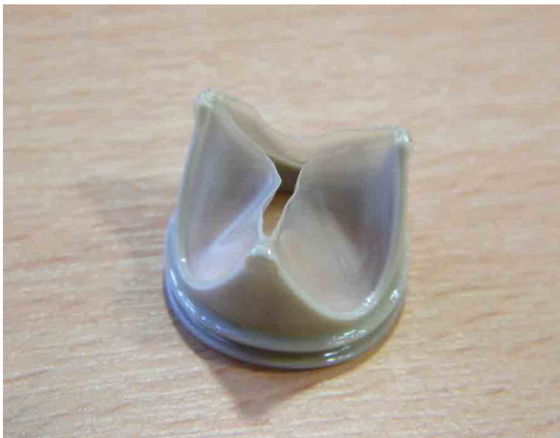
Figure 2 A replacement tri-leaflet heart valve made of various polymers. The leaflet is made of polyurethane whilst the frame of the heart valve is made of polyetheretherketone. The aortic valve is the gate between the main pumping chamber of the heart, the left ventricle, and the main artery of the body, the aorta. The aortic valve is able to open and close because it has leaflets (cusps). In a normal aortic valve there are three leaflets, and because of this it is called tri-leaflet.
