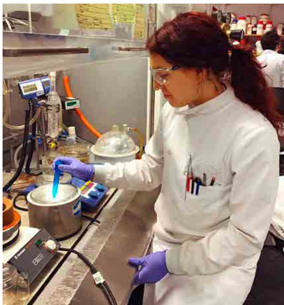
Figure 5 The author Amanda Pearce preparing a formulation of polymer nanoparticles loaded with the chemotherapeutic drug docetaxel. They are blue because they also have a fluorescent dye included for tracking by microscopy. Photo by Amanda Pearce
