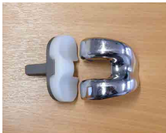
Figure 1 A knee implant with a polyethylene articulating surface (white component) between the femoral (upper leg bone) and the tibial (lower leg bone) components
