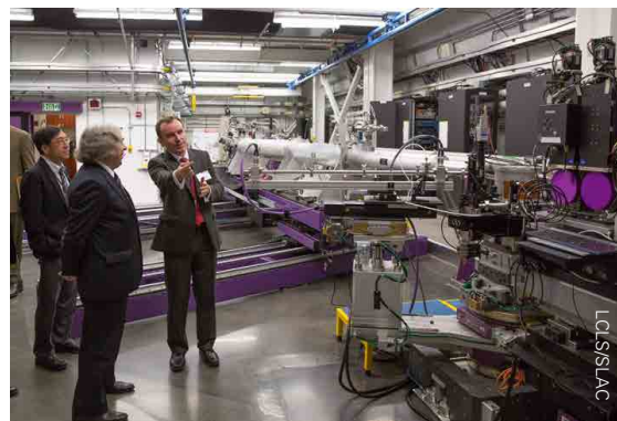
The X-ray Correlation Spectroscopy (XCS) experimental hutch is used to carry out experiments that observe dynamical changes of large groups of atoms. The SLAC director, Chi-Chang Kao (far left) and LCLS director, Mike Dunne (far right) can be seen in this picture.
