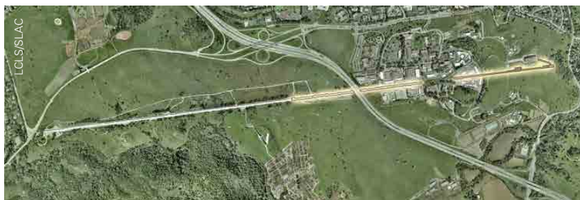
Bird's eye view of SLAC, where the highlighted region in the diagram is LCLS. The experimental hutches are the rooms to the far right of the image. The linear accelerator (linac) is on the far left and is the largest linac in the world.
