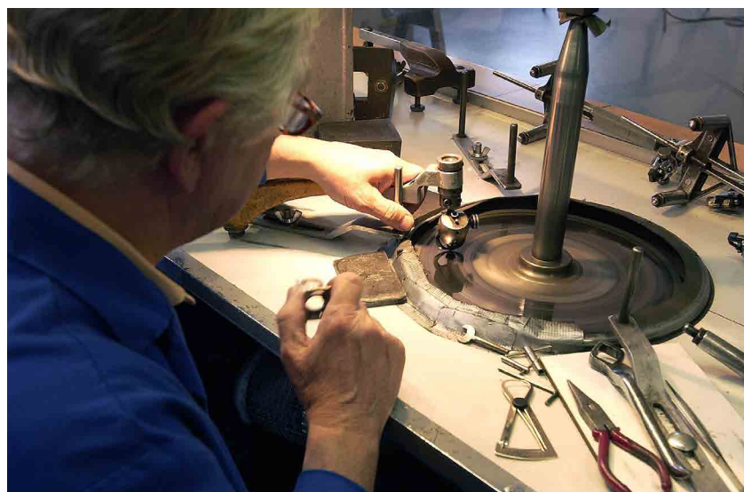
Computer modelling determines how best to cut a stone from a rough diamond. Hand polishing is still used to give the most brilliant surfaces.
