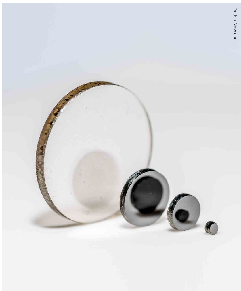
CVD-grown wafers of diamond (transparent, left) and boron doped diamond (black, middle, right).
