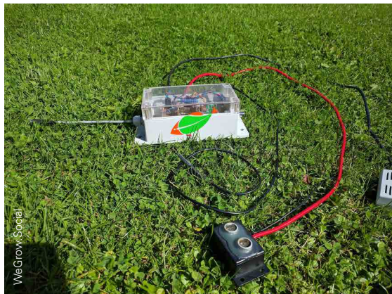
The WaterElf - a device that automatically monitors conditions in aquaponic systems
