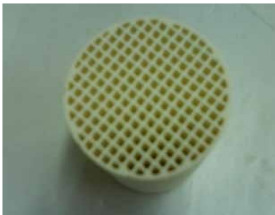
The honeycomb monolith in which the reactants meet the catalyst.
