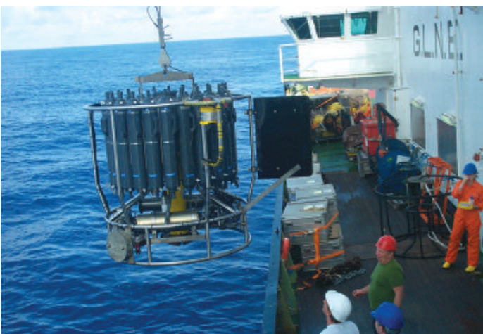
Above: The water samplers are lowered into the ocean Right: Stuart Cunningham working on a profiler before it is attached to a mooring cable (see back page)
