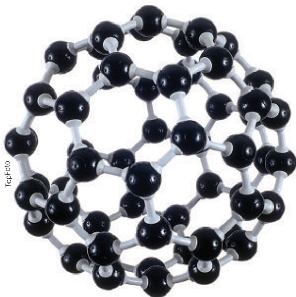
Figure 1 A buckyball. Nanotubes and buckyballs are nanoscale objects made of carbon atoms. They are likely to play an important part in electronic systems
