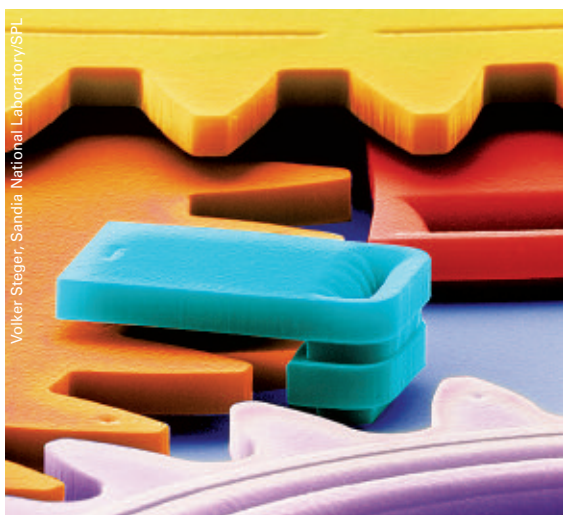
These miniature cogs and gears could form the basis of a microscopic machine. Machines on this scale are micromechanical, rather than nanotechnology. (The image was made using a scanning electron microscope; the colours were added later by computer)
