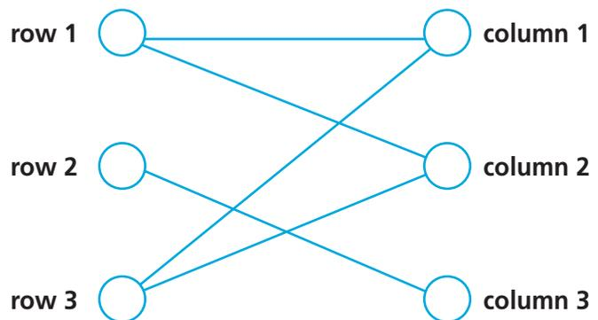
The graph lines are not all connected and so the attempted bracing fails.
