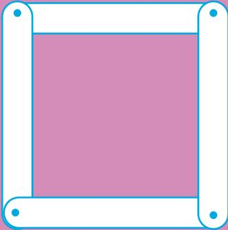
It can be made **rigid** by adding a single brace.
