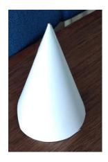
Fold a nose cone from A4 card and pack 50g of platicene inside
